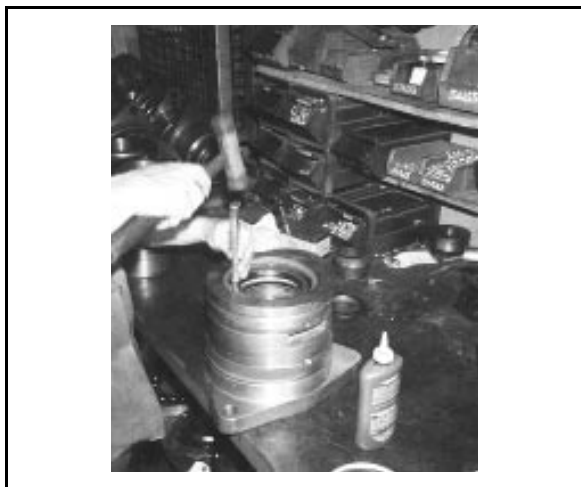
FIGURE 5 (MSSM0303AE) Installing Seals in Bearing Housing
